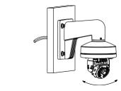
(3) Screw up and complete the fixation of adaptor
